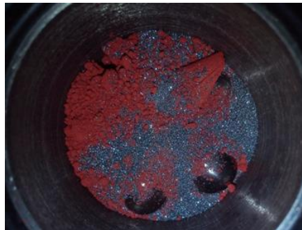
Fig. 1. Oxides in vial with iron balls
