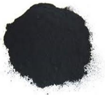
Fig. 2. \text{MnO}_2\text{-Fe}_2\text{O}_3 powders after 12 h milling
